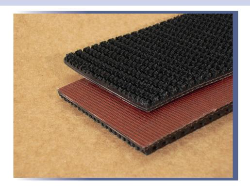
Rough top conveyor belt has been designed for transporting fragile or easily deformed goods such as glass, paper bags, carton boxes etc. and it can be used at angles up to 30 - 35 degrees, depending on the goods to be carried, in the range of temperature  $(-30...+70^{\circ}C)$ . The slip-resisting surface is ideal for steep inclined/declined applications. The carcass is made of polyamide / polyester (EP), polyester / polyester(EE), polyamide / polyamide (PP) fabrics.
