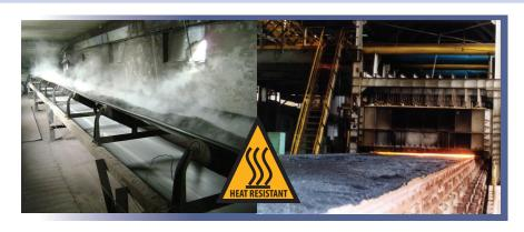
Heat can do a lot of damage to the carcass of the conveyor belt itself. It is very important to choose the right thickness of the covers because they act as a direct barrier between the heat source and the carcass. Basically, the thicker the covers, the better the protection it offers. Artego's **HEATSTOP** conveyor belts are specially engineered to convey sintered ore, hot pellets, hot clinker, hot chemicals, fertilizers, hot cement and many other materials.
